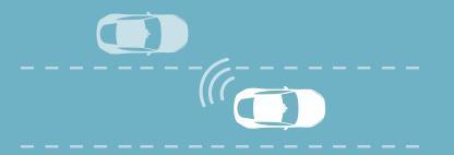
Blind Spot Assist Pack (Optional<sup>12</sup>) can help you prevent collisions. If another car is in your blind spot when you begin to change lanes, Blind Spot Assist detects the car and applies corrective torque to encourage you to guide your vehicle away from the approaching vehicle. Rear Traffic Monitor uses the same system to alert you, via the Touchscreen, of moving vehicles during reversing.
